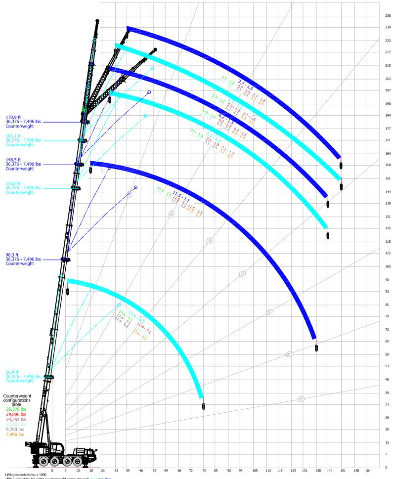
Lifting capacities for entire counterweight range shown in Cyan and Blue Lifting capacities for each counterweight configuration shown are color coded in aggrement with Counterweight configurations table
