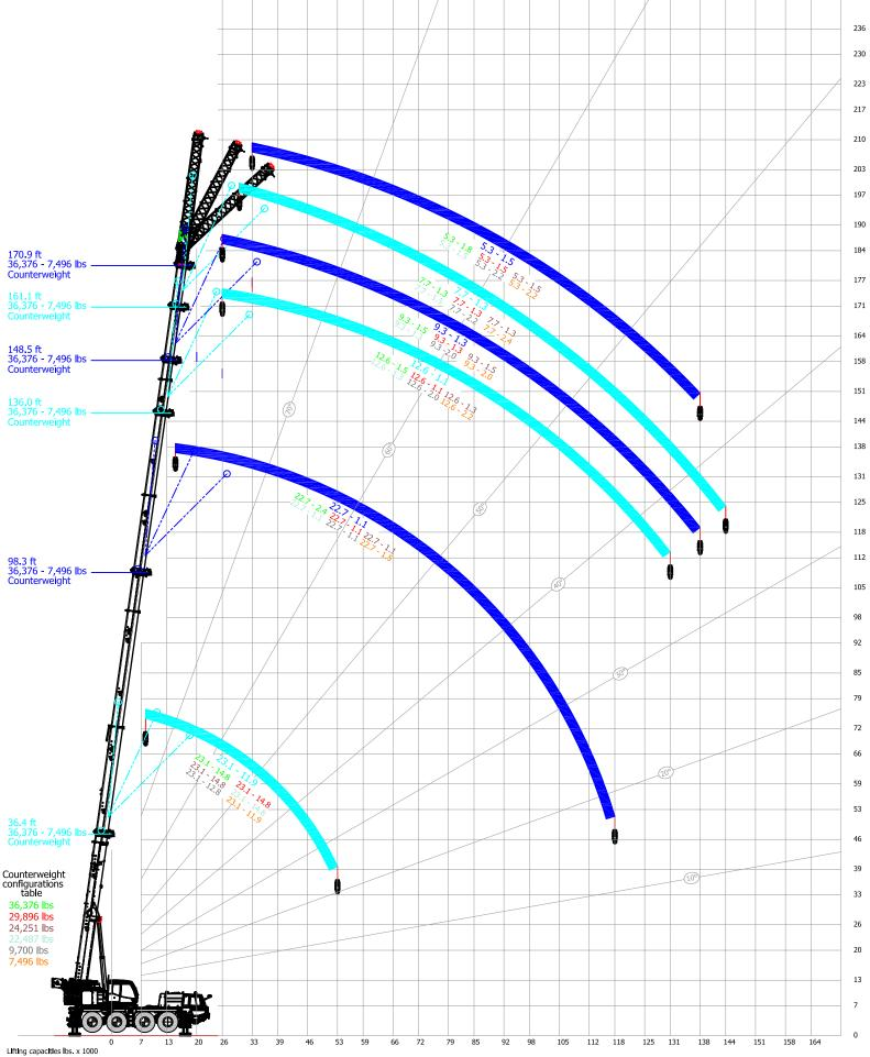
Lifting capacities for active counterweight range shown in Cyan and Blue Lifting capacities for each counterweight configuration shown are color coded in aggrement with Counterweight configurations table
