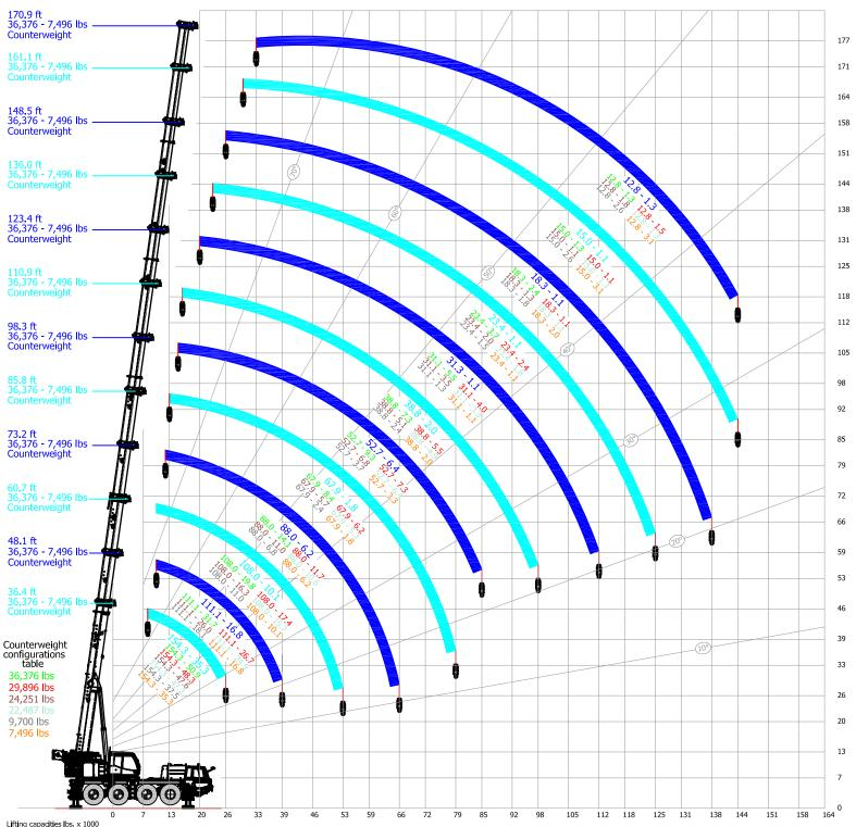
Lifting capacities for entire counterweight range shown in Cyan and Blue Lifting capacities for each counterweight configuration shown are color coded in aggrement with Counterweight configurations table
