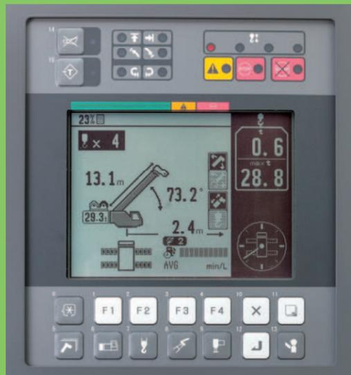
Tadano's new AML-C is easy to use. It allows the operator to simultaneously monitor: boom angle, boom length, elevating cylinder operating pressure, the extended length of the outriggers, swing position, rated lifting capacity and present hook weight. All of this enables the AML-C to move easily through lifting capacity changes without changing configurations and codes to make a lift.
