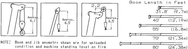
supporting surface. Boom deflection and subsequent radius and boom angle change must be accounted for when applying load to hook.
