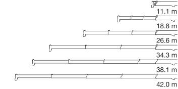
The above lifting height and boom angle are based on a straight (unloaded) boom and machine standing level on firm supporting surface. Allowance should be made for boom deflection obtained under loaded conditions. The above working range is shown on condition with outriggers fully (7.0 m) extended.
