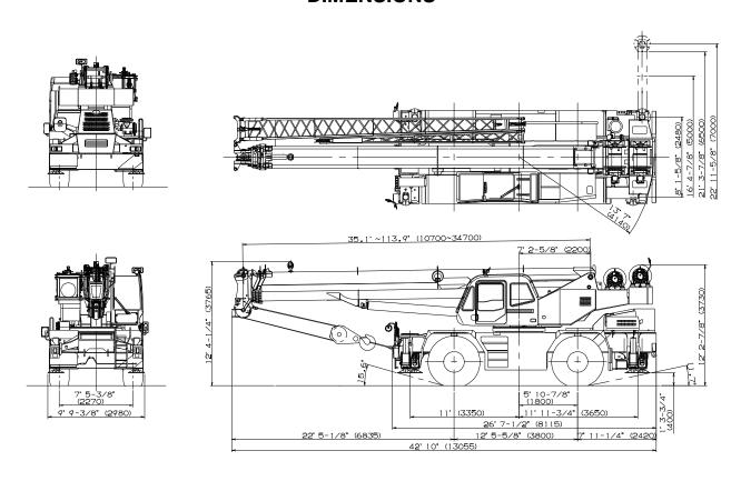
Note: Dimension is with boom angle at -0.8 degree.
