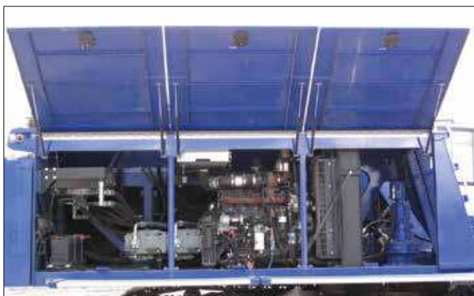
Large access doors, spacious machinery compartments simplify preventative maintenance and service of the crane.
