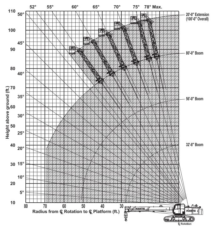
Limits of operation: Maximum load capacity = 750 lb Maximum radius when mounted on main boom = 68 ft
