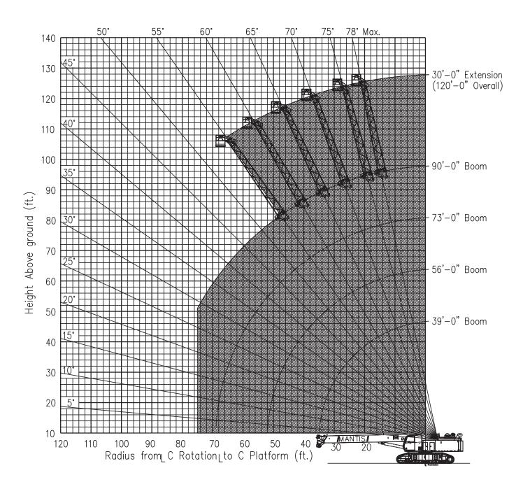
Limits of operation: Maximum load capacity = 750 lb
