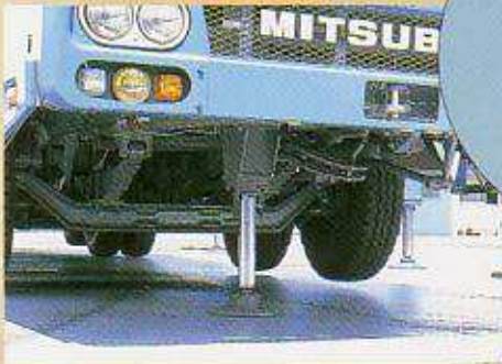
By attaching a front (fifth) jack, full lifting capacity is achieved through a 360° swing.
