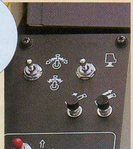
A special switch on the control lever makes it possible to control twin swing easily.
