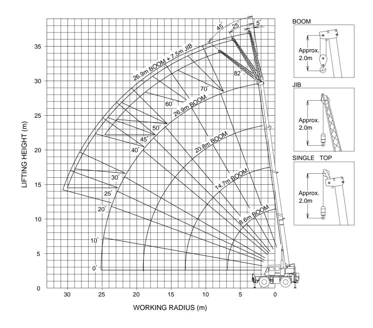
**NOTE :** The above lifting heights and boom angles are based on a straight (unladen) boom, and allowance should be made for boom deflection obtained under laden conditions.
