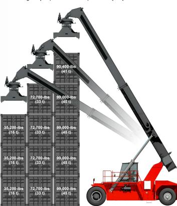
Rated Container Capacity 99,000-lbs. (45 t) First Row / 4-high Stacking 9.5-ft. (2.9 m)
