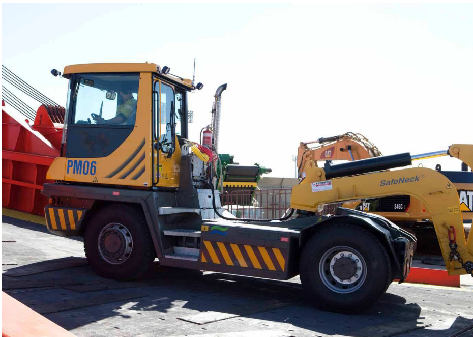
The SafeNeck provides improved stability and extra safety during RoRo ramp operations.
