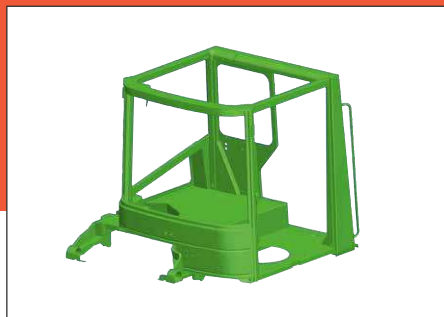
All-steel cab structure (FOPS and ROPS tested)
