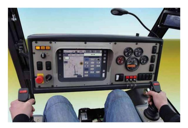
Crane operators looking for a well-designed control system — and, of course, a comfortable seat — will find exactly what they want on Terex® all terrain cranes. The touchscreen interface is standard on nearly all Terex® all terrain cranes, including the ability to customize the configuration for the preferences of the operator. The ergonomic working environment has all controls within easy reach, helping operators to stay focused on the job rather than searching for controls.
