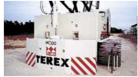
Hydraulic removable counterweight system
