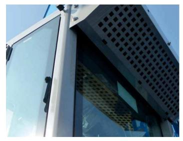
Air conditioningDust-protected, separated from the main cooling system
