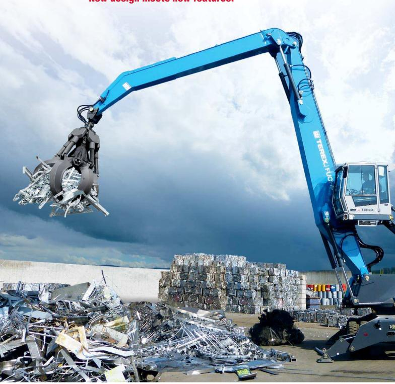
The MHL350 F material handler sets the standard in modern technology with more sophisticated hydraulics and an exceptionally comfortable driver's cabin.
