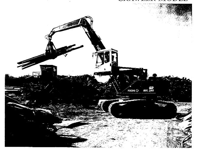
Track width hydraulically adjustable provides ease of transport plus great stability Large windows and ergonomic cab add to visibility and operator comfort Elevating cab adds to machine flexibility
