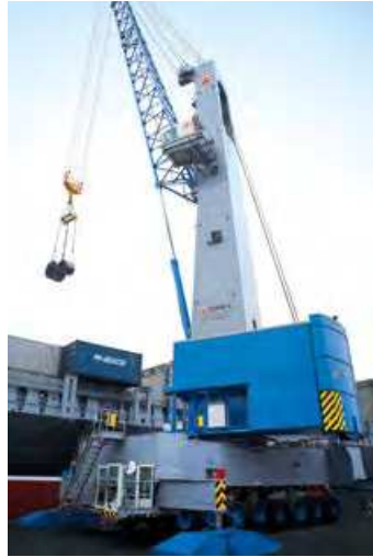
Terex® Gottwald Model 7 harbour cranes: handling containers, general and project cargo as well as bulk materials with motor or four-rope grab.
