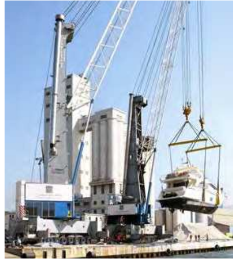
Terex® Gottwald Model 7 harbour cranes: handling containers, general and project cargo as well as bulk materials with motor or four-rope grab.
