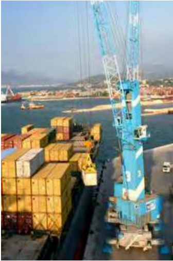
Terex® Gottwald Model 7 harbour cranes: handling containers, general and project cargo as well as bulk materials with motor or four-rope grab.
