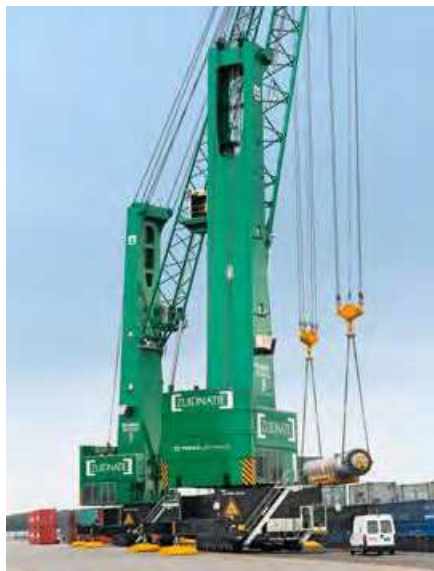
Terex® Gottwald Model 8 harbour cranes: Handling containers, general and project cargo as well as bulk materials with motor or four-rope grab.
