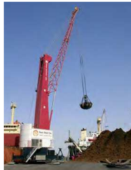
Terex® Gottwald Model 8 harbour cranes: Handling containers, general and project cargo as well as bulk materials with motor or four-rope grab.
