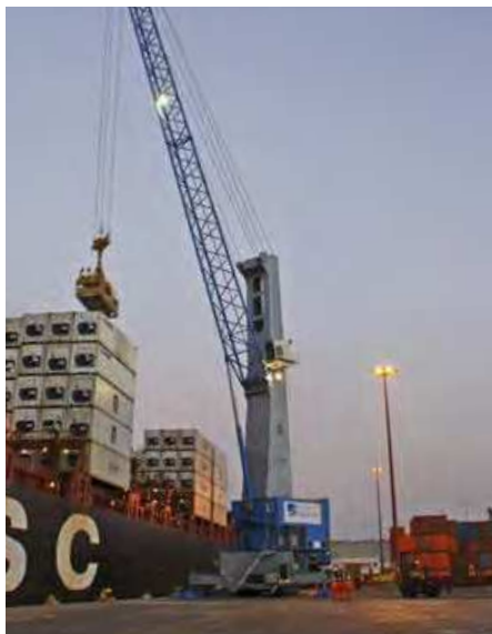
Terex® Gottwald Model 8 harbour cranes: Handling containers, general and project cargo as well as bulk materials with motor or four-rope grab.
