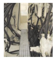
The front section of the walk-through engine module allows easy access to major hydraulic components, e.g. pumps, filters and swing drives.
