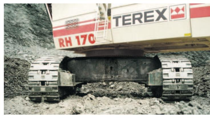
Backed by longstanding experience in rugged mining operations, TEREX O&K developed for its RH 170 an undercarriage that sets new standards in robustness and reduced maintenance. Special attention was directed at optimizing the flow of forces and the service-life of the crawler components. Wear zones were minimized, track pad geometry refined and wear area cross-section enlarged.
