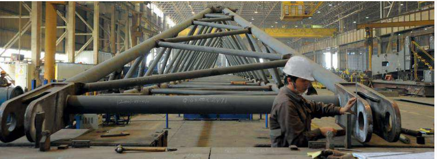
Manufacture of lattice booms for the Quaymate M50 mobile harbour crane in Xiamen, China
