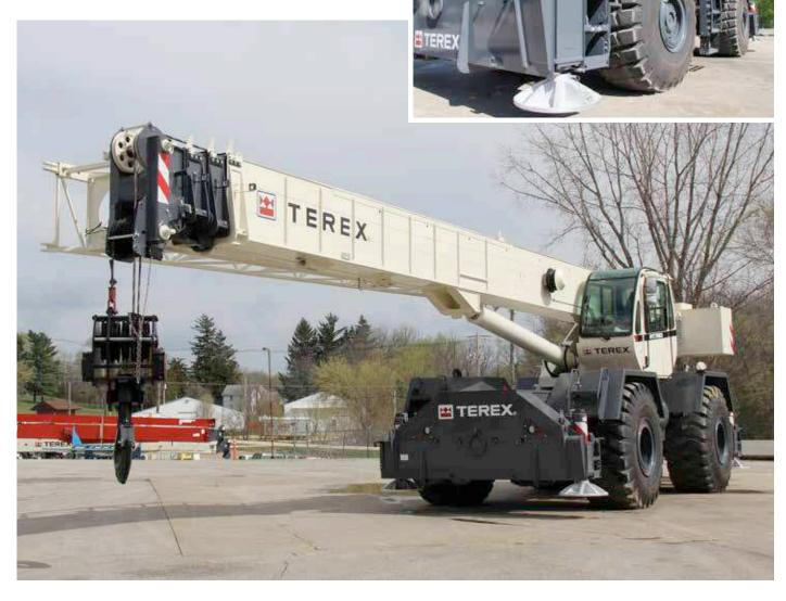
Both the weight and width of Terex Rough Terrain Cranes are optimized for on-road truck transport. On the jobsite, you can select the travel speed you need from a powershift transmission and steer by selecting from three steering modes. You'll increase your productivity on the job.
