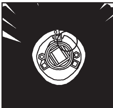
FIGURE 4 Improper Placement of Drive Pins (Circled)
