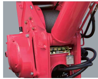
9 Automatic stop for leaving minimum wire rope
