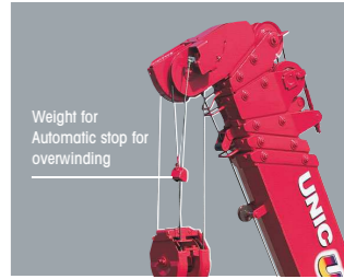
8 Automatic stop for overwinding
