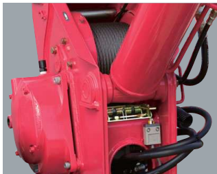
9 Automatic stop for leaving minimum wire rope
