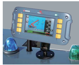
7 Safe load indicator
