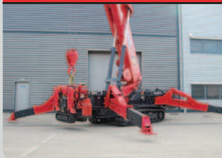
Outriggers extended for stability
