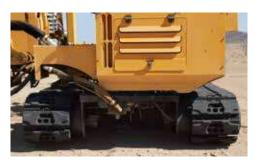
LEAVE IT LIKE YOU FOUND IT. The PD10 features a wide track pad to minimize jobsite disturbance in widely varying ground conditions.
