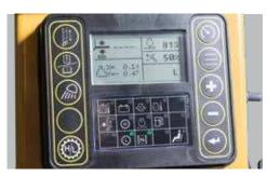
AT YOUR FINGERTIPS. An industry-unique integrated control system offers the operator a variety of machine information, including pile angle and height. Display also shows machine maintenance information to help maintain service schedules.
