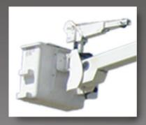
Bucket capacity: 700 lbs (with jib installed)/800 lbs (without jib installed)
