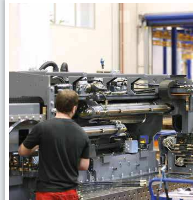
During final assembly, VÖGELE screeds undergo a variety of functional tests.
