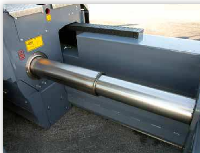
The VÖGELE single-tube telescoping system guarantees maximum stability even when the screed is set to its maximum width.
