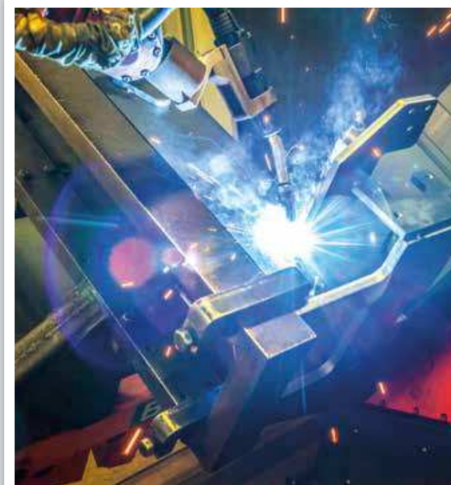
Welding cell for screed frames. Robot-produced weld seams feature consistent, high quality and precision.
