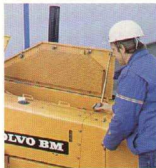
The radiator grille can easily be swung out for cleaning.
