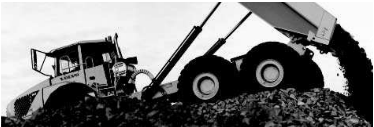
Load & Dump brake is activated with a single press of a button.
