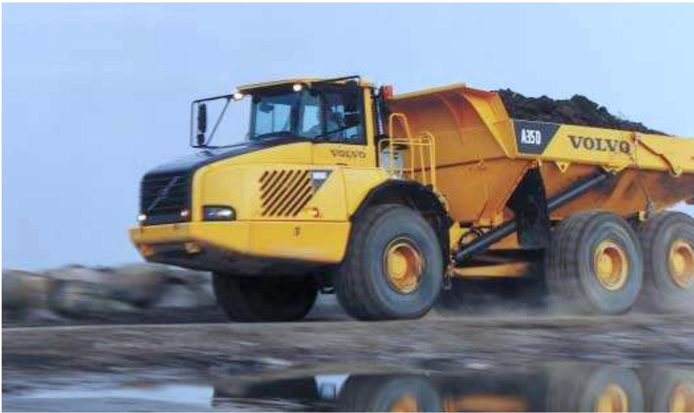
The front axle's sturdy rubber suspension with shock absorbers means that it can maintain high average speeds while preserving operator comfort and minimizing mechanical wear. The bogie design means that each pair of wheels can move independently to maintain ground contact. This lets the body move practically horizontally over irregularities in the ground while the frame undergoes less stress.
