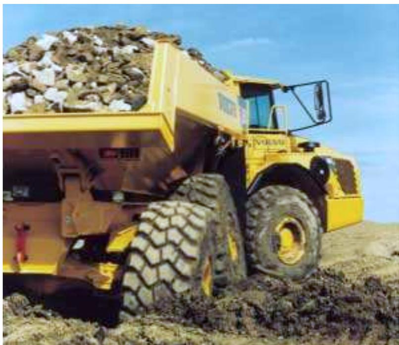
*The self-compensating hydro-mechanical steering gives steering comparable to a passenger car.*
