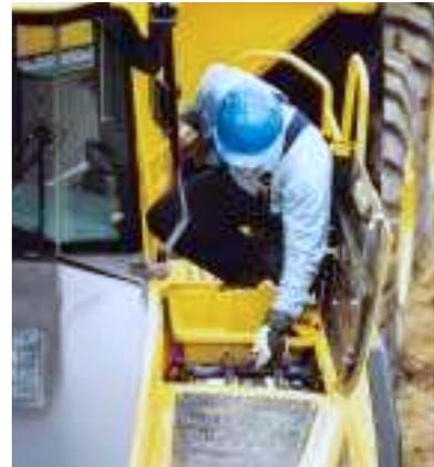
*The batteries are easily accessed next to the storage compartment.*
