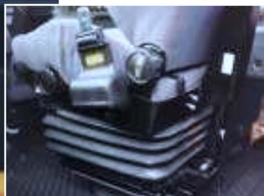
*An air suspension operator's seat improves comfort.*
