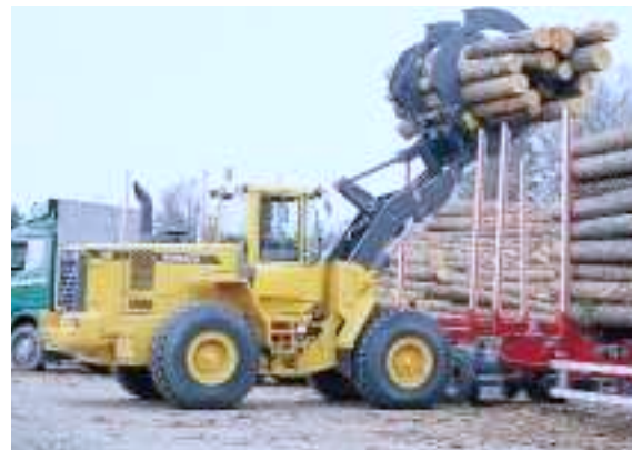
TP linkage comes into its own in logging applications. No other system can provide such high breakout torque throughout the entire lift cycle.
