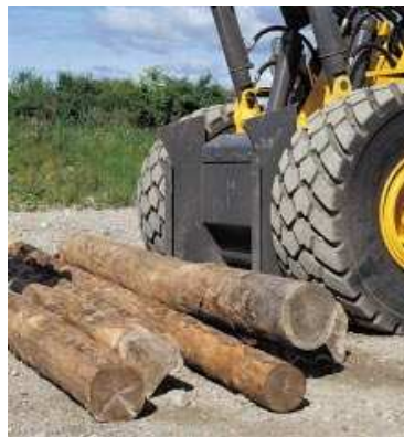
With log pusher and kick-out you can build higher stacks and utilize the storage space on the wood yard more efficiently.
