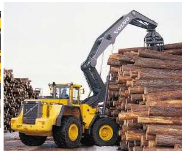
With log pusher and kick-out you can build higher stacks and utilize the storage space on the wood yard more efficiently.
