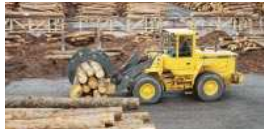
The long wheelbase and compact lift-arm geometry provide the necessary stability for timber handling with a tree-length grapple.
