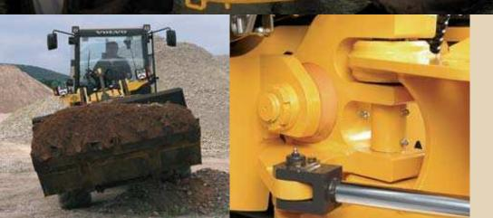
• Articulating oscillating joint for optimum manoeuvrability.
