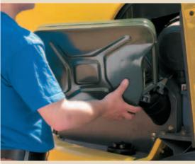
Easy fuel filling, even directly form a fuel can without spout of funnel.
