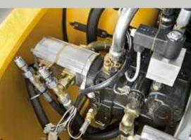
· Separate working and steering hydraulic pumps.
