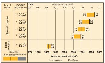
The size of rock buckets is optimized for optimal penetration and filling capability rather than the density of the material.
