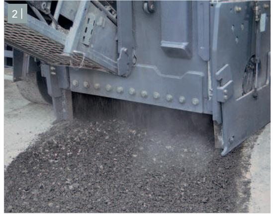
1 | - 2 | *Hydraulically height-adjustable scraper blade*
