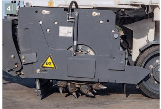
3 | - 4 | *When fully lowered, the hydraulically adjustable edge protector reliably closes the drum housing while enabling the cold milling machine to be driven along obstacles when raised.*
