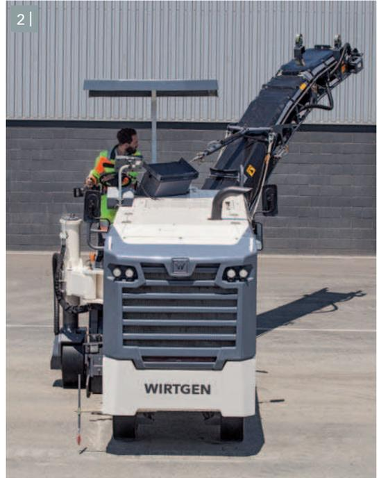
1 | - 2 | Flexibility is ensured by wide conveyor slewing angles.
