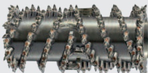
Standard milling drum Milling width: 6 ft. 6 in. (2,000 mm) Milling depth: 0-13 in. (0-330 mm) Tool spacing: (15 mm)
