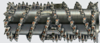
Standard milling drum Milling width: 7 ft. 2 in. (2,200 mm) Milling depth: 0-13 in. (0-330 mm) Tool spacing: (15 mm)
