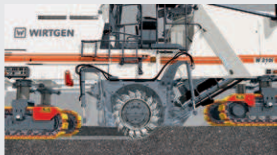
4 | Cold milling machine mills at full working depth right from the first metre
