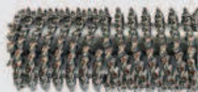
Fine milling drum Milling width: 2,000 mm Milling depth: 0-100 mm Tool spacing: 8 mm
