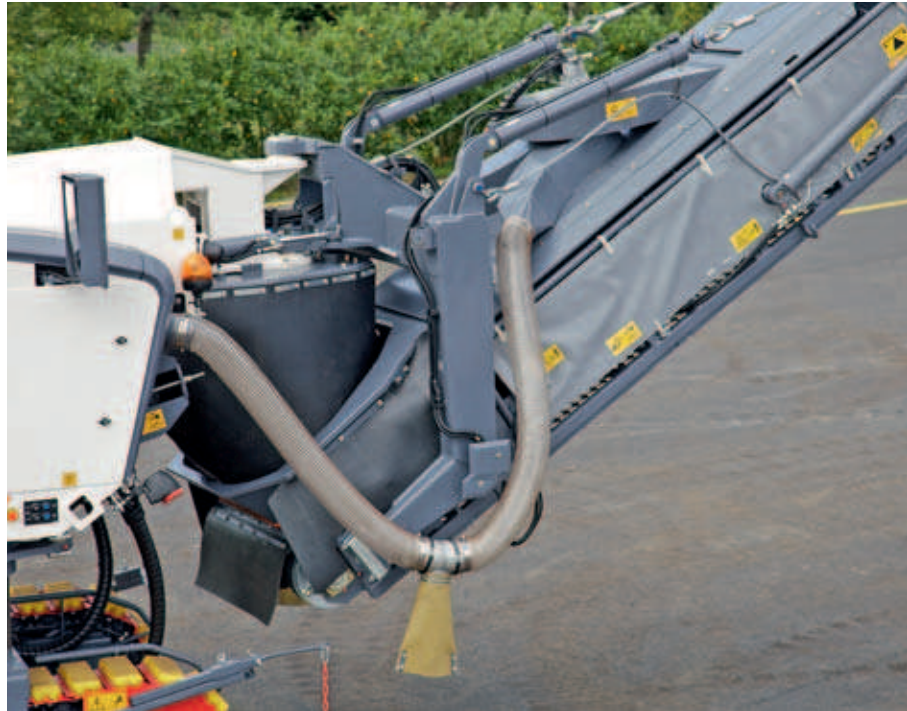
The centrifugal fan can be adjusted in speed.
