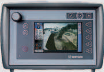
2 | Camera at end of conveyor
