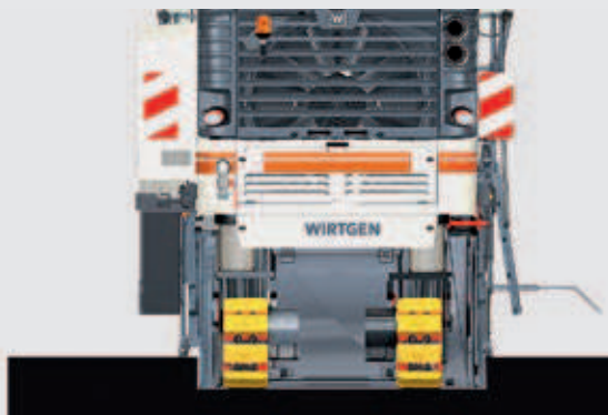
W 250i with 2.2-m drum assembly
