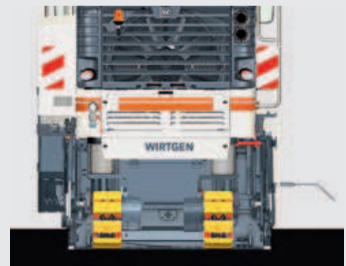
W 250i with 2.5-m drum assembly
