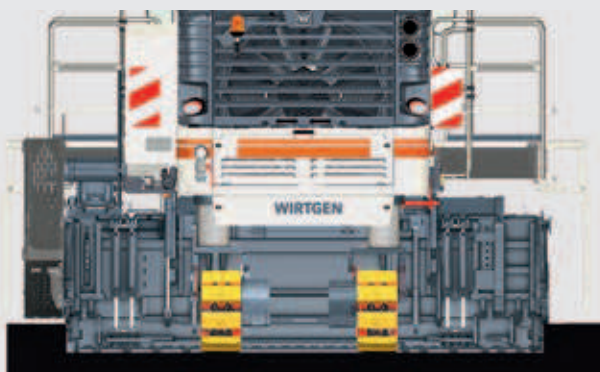
W 250i with 3.8-m drum assembly
