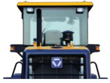
Full-view rear window, high mounted rear lamp and equipment for reverse alarm provide good vision and safe
