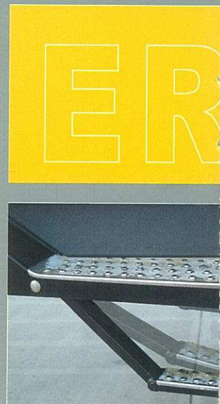
脚踏板(遇障碍可自动收起) step plate(auto stowing by encountering obstacle) Courtesy of CraneMarket
