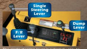
The single steering lever is extremely easy to operate with one hand. The easy controls give the operator hours of low-fatigue operation.
